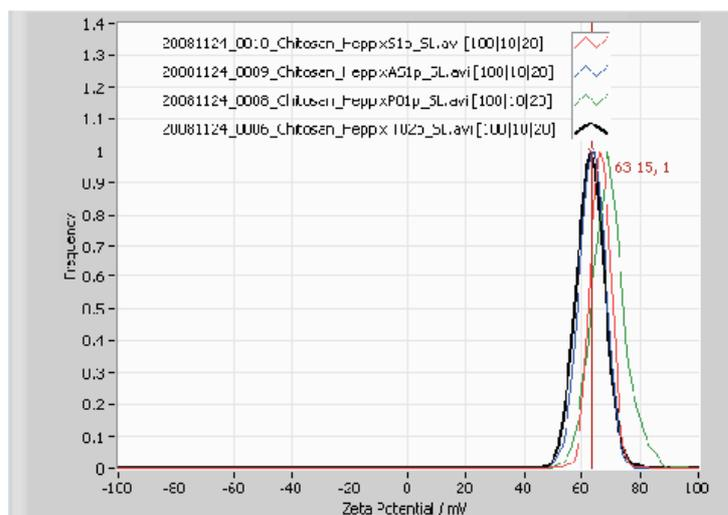
To make sure, that the results obtained with the ZetaView® are reasonable, titrations with charge calibrated anionic PVS solutions were performed in the Stabino®. The end point was 0 mV. It is known that the streaming potential at the starting point as well as the consumption of counter polarity poly-electrolyte to the zero point of charge correlate to the zeta potential. As in the ZetaView® particle tracking analyzer, the results on the same 4 samples showed a high potential and the same trend.
