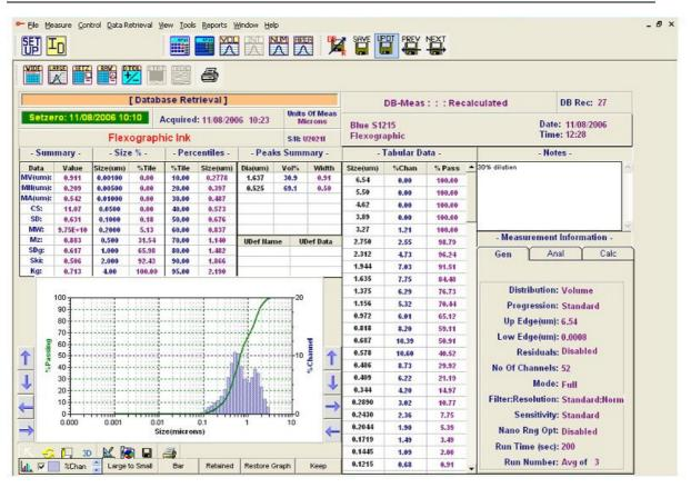
In the second figure, a comparison is provided for FLEXOGRAPHIC blue ink with magenta. The comparative graph was developed using Particle Metrix FLEX software which allows direct copying into PowerPoint. The magenta sample does not show the presence of a second distribution mode by either NANO-flex® or microscopy.
