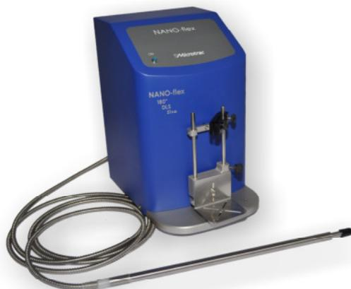
At LLT (Chair for laser technology) in cooperation with Interactive Materials Research DWI (German institute for wool research at RWTH Aachen e.V.) a Nanotrac® size measurement instrument was purchased to track the synthesis of microgels by precipitation polymerisation in a reactor (Figure 2) at varying process conditions.
